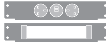
Option 3: 2x GPO - Type G** 2x USB Power 200mm Data Provision
