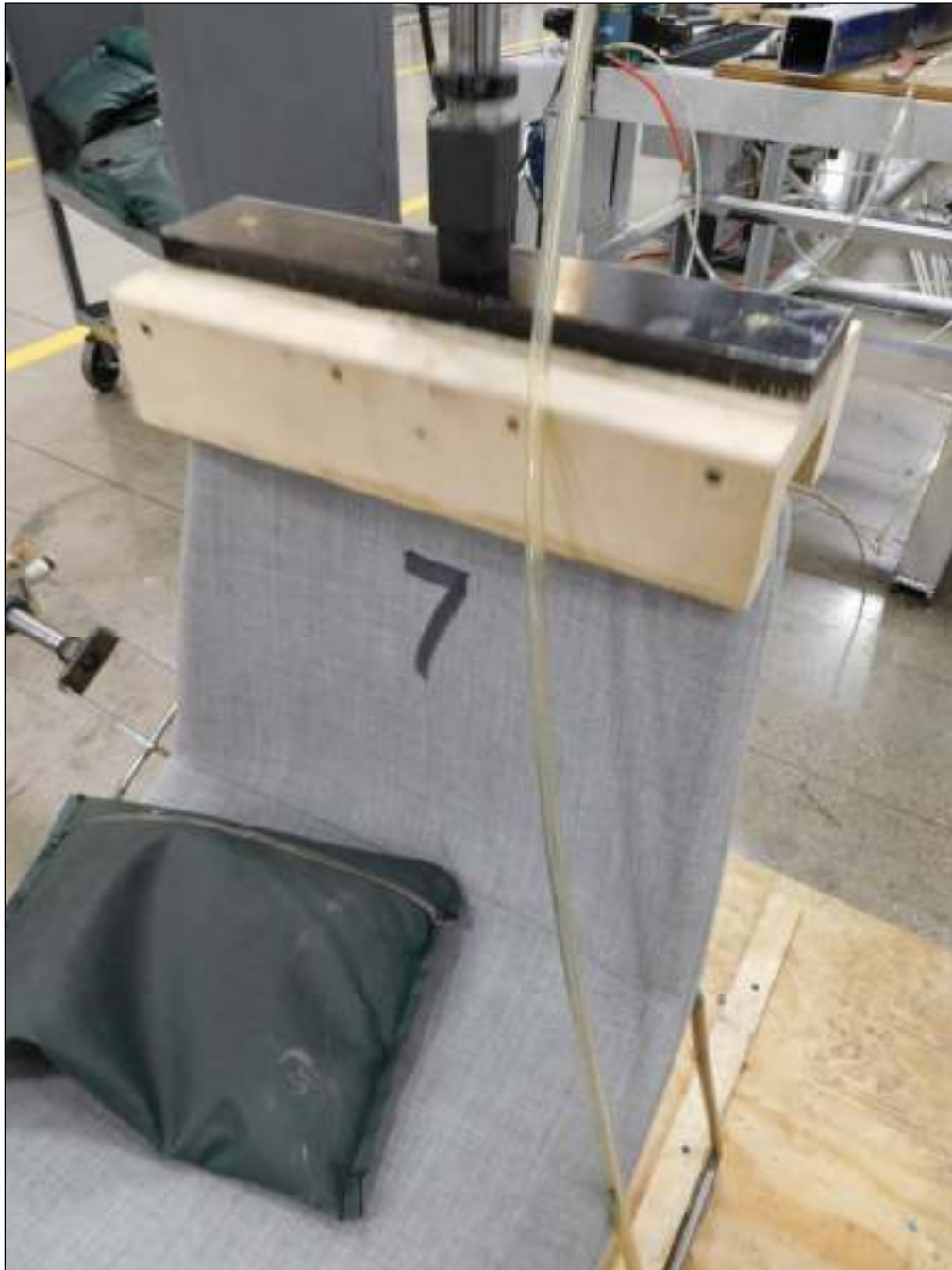
Vertical Back Durability - Cyclic
