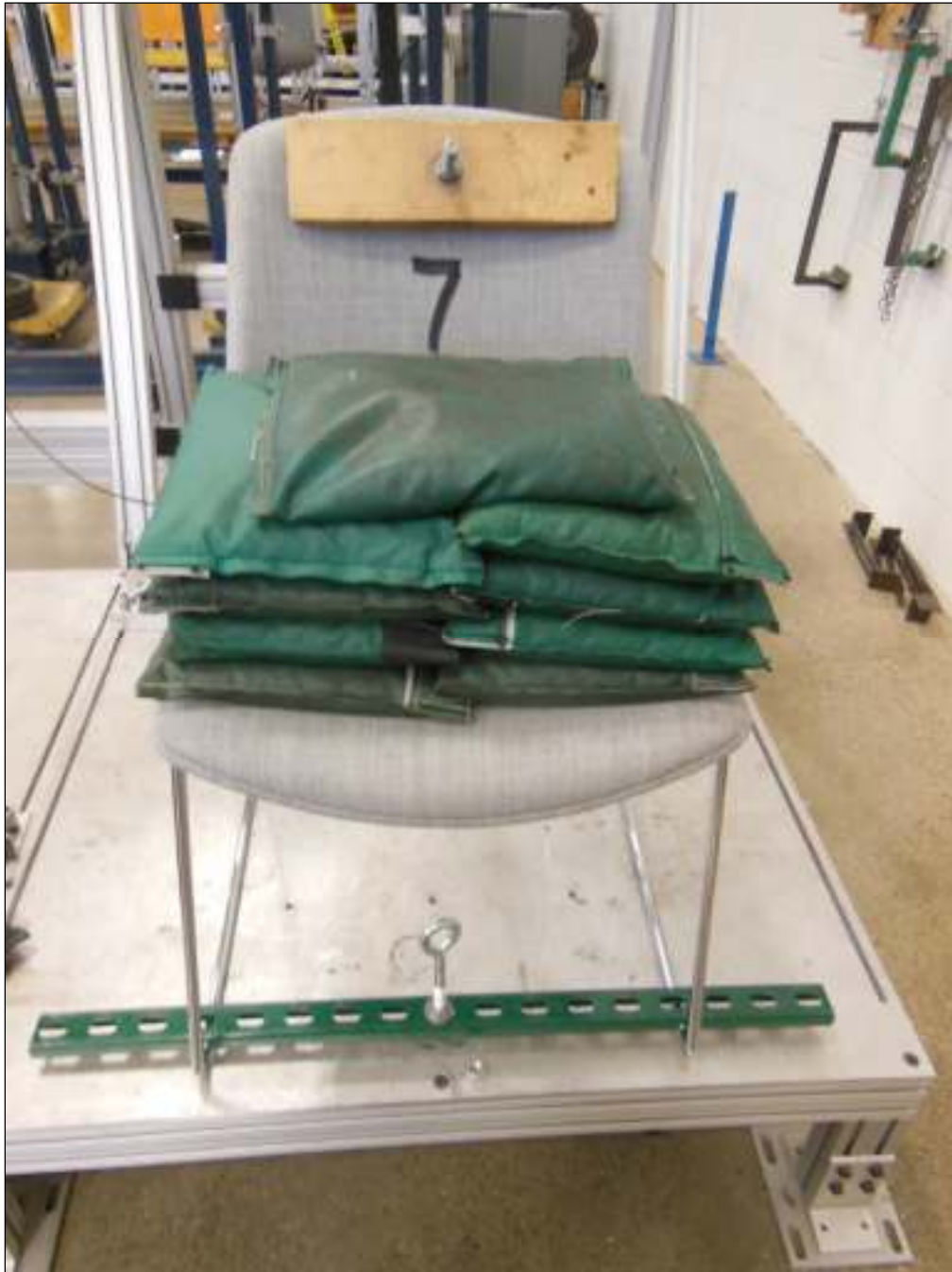
Horizontal Back Durability - Cyclic
