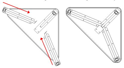
3. Secure the three legs together <u>loosely</u> with the connector bolt provided.
