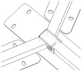
4. Fasten the frame assembly to the top using the screws provided. Finally, tighten the connector bolt using the allen key (hex key) provided.
