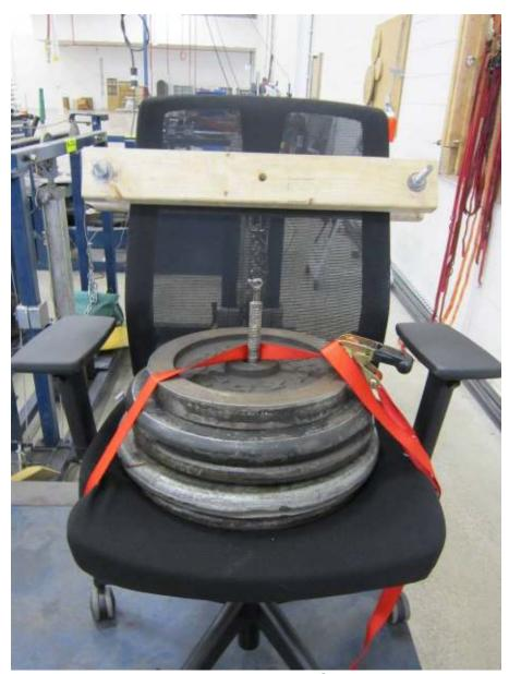
Tilt Mechanism Test-Cyclic
