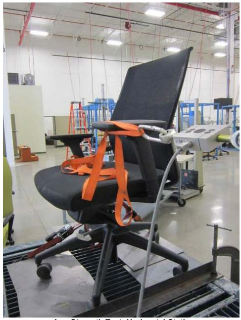
**Arm Strength Test- Horizontal-Static**
