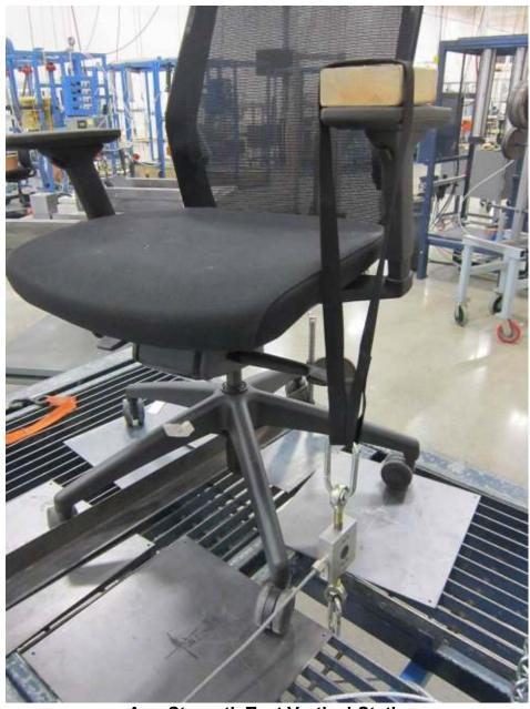
**Arm Strength Test Vertical-Static**
