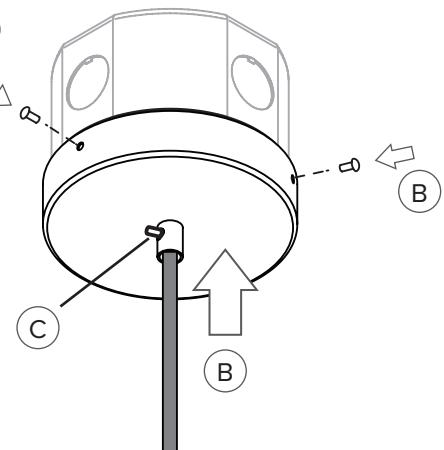
Place canopy cover over canopy base and fasten grub screws (B). Adjust power cable and fasten grub screw on strain relief (C). (Levez le pavillon en position et ressérez les vis (B). Ajustez la bride de décharge(C).)
